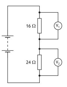
The reading on voltmeter  $\rm V_1$  is 3.6 V.
