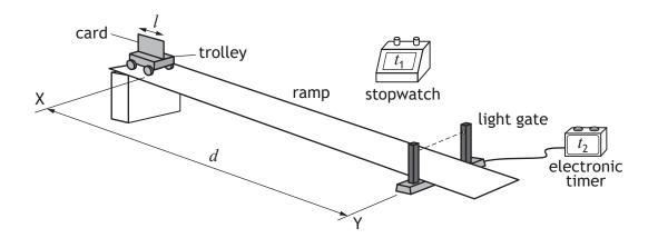
The trolley is released at X and travels down the slope.
