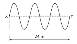
The speed of the wave is  $48 \text{ m s}^{-1}$ .
