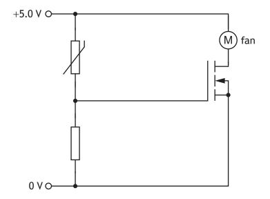
As the temperature of the charger increases, the resistance of the thermistor decreases.
