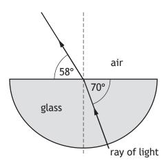
Which row in the table shows the angle of incidence in the glass and the angle of refraction in air?
