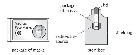
(a) The gamma radiation is produced by a cobalt-60 source.
