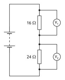
The reading on voltmeter  $V_1$  is 3.6 V.
