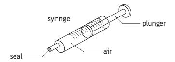
The initial volume of the air in the syringe is  $1.40\times10^{-6}~\text{m}^3$  and the pressure is 120 kPa.
