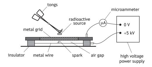
A radioactive source is placed close to the metal grid.
