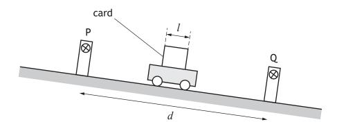
The time taken for the card to pass through light gate P is  $t_1$ .
