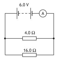
(i) Calculate the total resistance of the circuit. Space for working and answer
