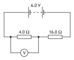
Calculate the reading on the voltmeter.
