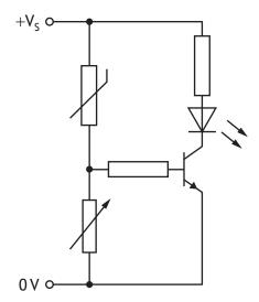
The variable resistor is adjusted until the LED switches off.
