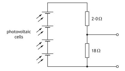
In direct sunlight the photovoltaic cells produce a combined voltage of 4.0 V.
