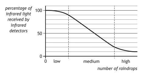
The percentage of infrared light received by the infrared detectors from the LEDs controls the frequency with which the windscreen wipers move back and forth.
