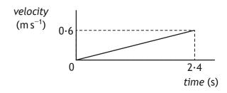
Determine the distance travelled by the trolley in the first 2.4s after its release.
