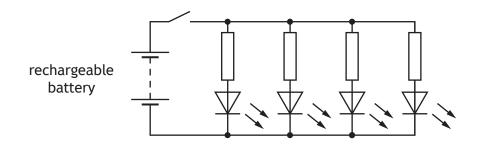
The switch is now closed and the LEDs light.
