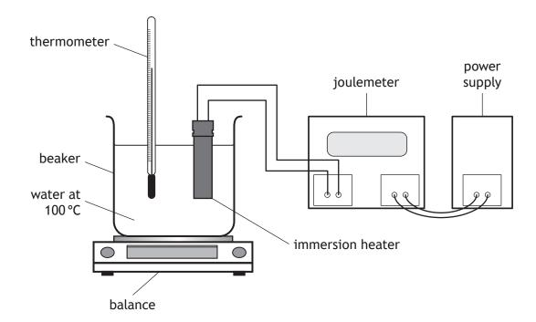
Describe how this apparatus would be used to determine a value for the specific latent heat of vaporisation of water.
