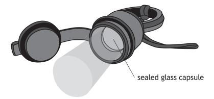
Beta particles emitted by the tritium gas are absorbed by a coating on the inside of the glass capsule.
