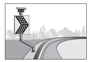
The warning sign uses a number of LEDs powered by solar energy.
