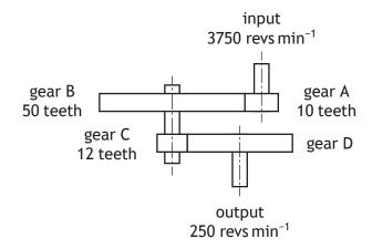
(c) Calculate the number of teeth on gear D.
