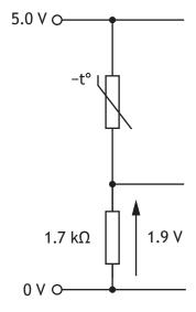
(b) Calculate the resistance of the thermistor for the condition shown above.
