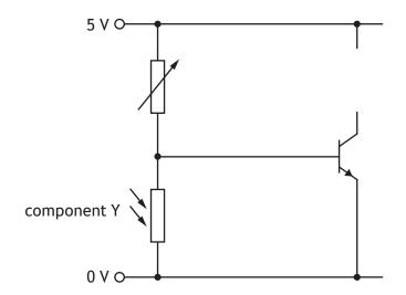
(a) Complete this circuit diagram by adding the symbol for the lamp.
