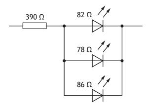
(i) Calculate the resistance of the three LEDs in parallel. (d)
