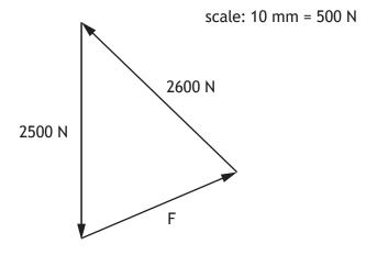
(c) Determine, with reference to the triangle of forces diagram, the size of unknown force F.
