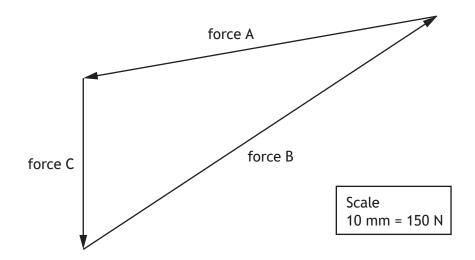
(a) Determine, with reference to the triangle of forces, the size of force A.
