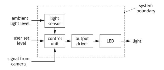
(a) Describe the purpose of the system boundary in a sub-system diagram.
