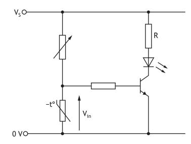
(c) Describe the operation of the circuit as the temperature increases.
