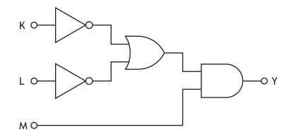
(f) Complete the Boolean equation, in terms of inputs K, L and M, for this logic diagram.
