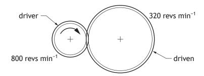
(a) Calculate the velocity ratio of this simple gear train.
