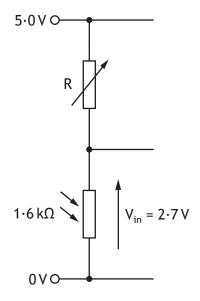
(e) Calculate the resistance of the variable resistor (R) for the condition shown above.
