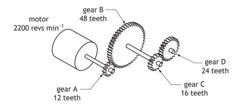
(b) Calculate the output speed of gear D.
