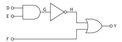
(e) Complete the truth table for this logic circuit.
