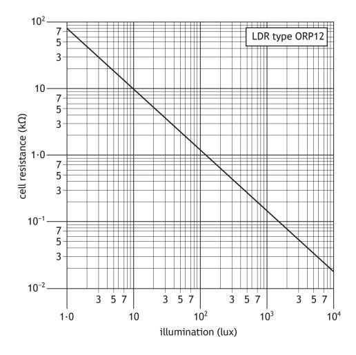
(f) Determine, with reference to the graph, the illumination level when the LDR has a resistance of  $200\,\Omega$ .
