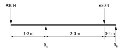
(a) (i) Calculate the reaction force  $R_{A}$  by taking moments about  $R_{B}$ .
