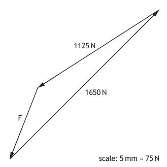
(c) Determine, with reference to the triangle of forces shown, the unknown force F.
