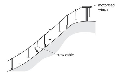
A motorised winch which is rated at 230  $\rm V$ , 12  $\rm A$ , is used in the operation of the tow.
