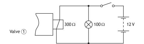
(c) Calculate the total resistance of the circuit.Show all working and final unit.
