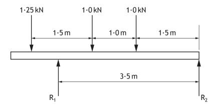
(e) Calculate the size of reaction force R<sub>1</sub>, by taking moments about R<sub>2</sub>.Show all working and final unit.
