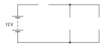
2. An electric torch is shown in the diagram below. The lamp is rated at 7.2V and 0.7A.
