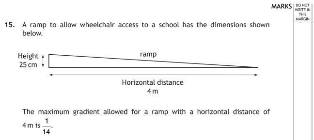
Does the gradient of this ramp meet the regulations?
